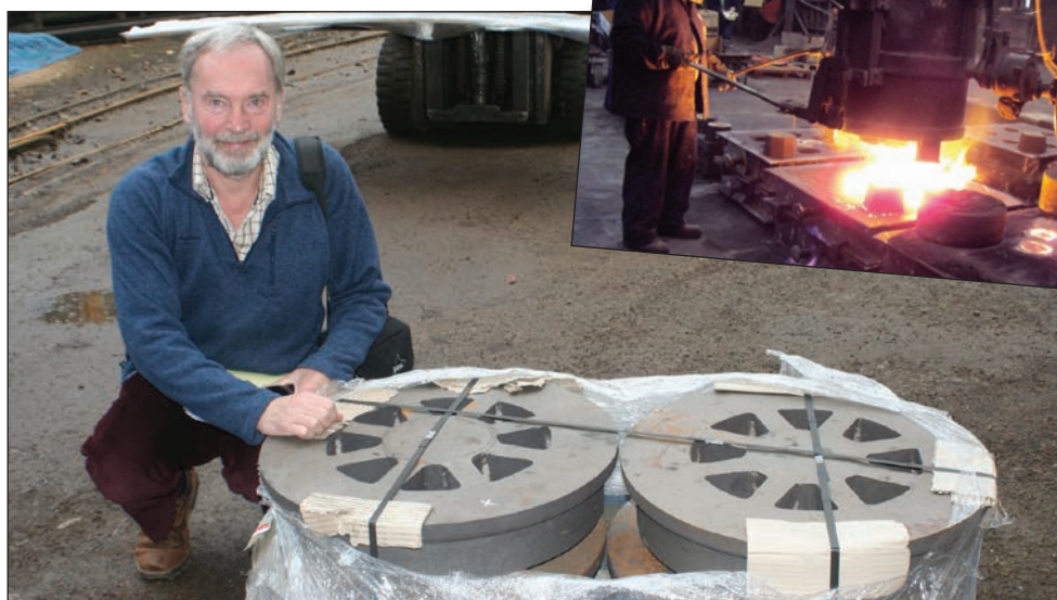
Below: Like the driving wheels (inset) the wheels for the leading and trailing trucks have been cast and are seen here with Technical Director Peter Best after arrival at Alan Keef & Sons. Photo: Andrew Charman
