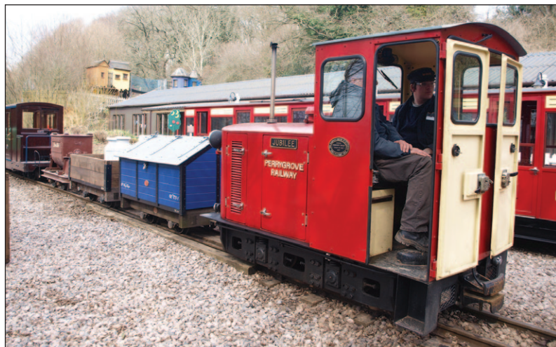
The 1994-built four-wheel diesel-hydraulic 'Jubilee' is a very easy-to-control yard shunter, as David Williams here discovers.
