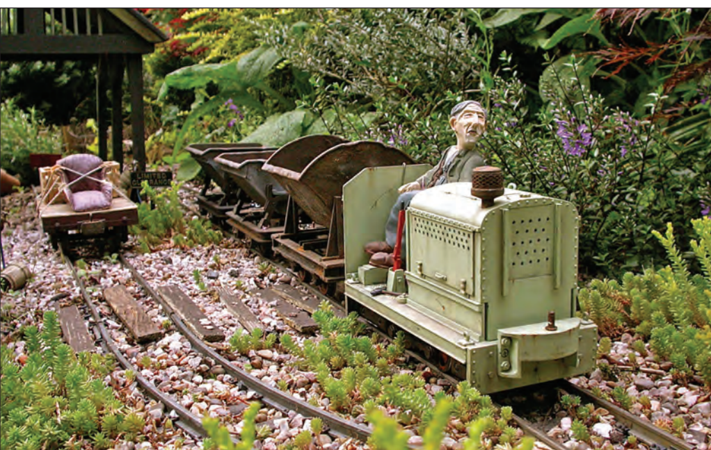
Left: Possibly the most gorgeous live steamer I have ever seen, our cover star, Rob Bennett's Salopia is a Simply 7/8ths 'Baldrig' body kit on an Accucraft 'Edrig.' Rob added much extra detail, which is topped off by an impeccable paint job commissioned from Si Harris. Note the DJB working scale resonator whistle on the spectacle plate. Photo: Rob Bennett
