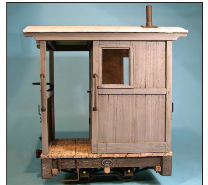
Right: Each year the 7/8ths Lounge runs a secret Santa-style car swap. Si Harris built this Way Car for last year's, in oak and pine over a set of resin test castings for a Western Wheeled Scraper style chassis. Various details include a brake wheel and ratchet, along with lamp irons from Talisman Castings, steps from Ozark and grab handles from Mamod. Photo: Si Harris
