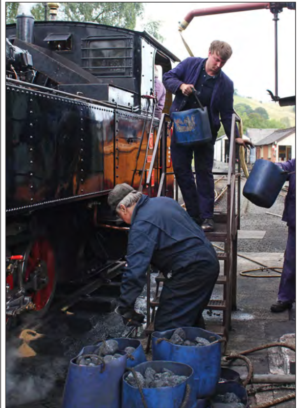
Above: On the ZB2 coaling up the bunker is not the easiest of tasks...
