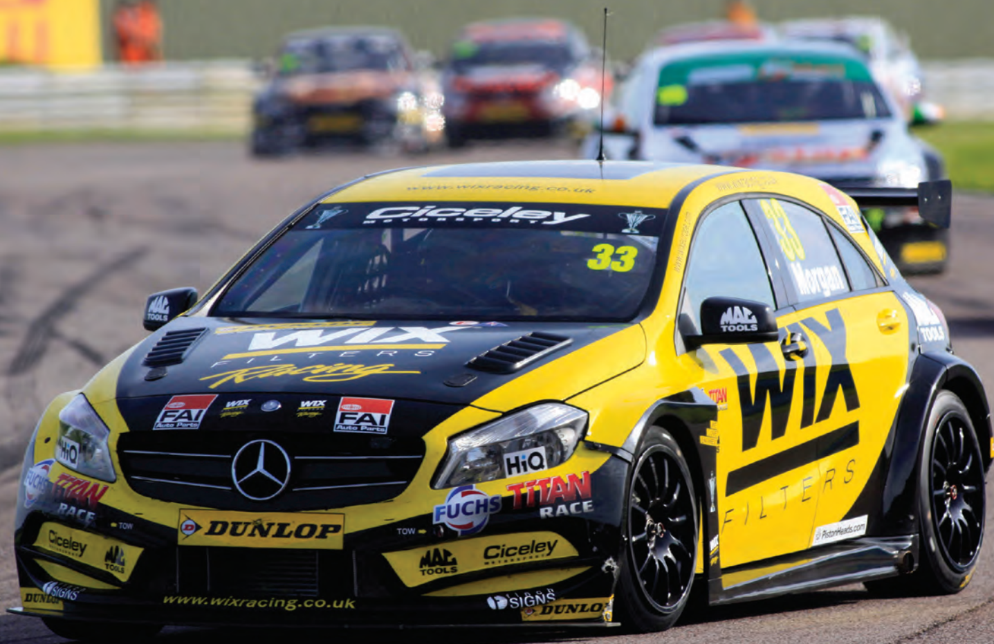
ABOVE Identity change: Adam Morgan's Mercedes A-Class is a prime example of the BTCC NGTC formula's flexibility – most of its components spent the 2013 season in a Toyota Avensis shell
